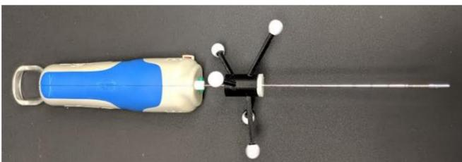
Figure 1. Biopsy needle with 3D-printed holder for infrared markers.
