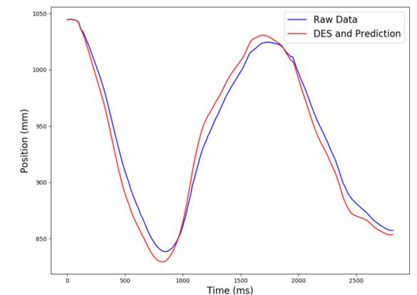
Figure 5. Example of double exponential smoothing and prediction for z position. Smoothing and prediction are applied to x, y, and z position, as well as to the quaternion. This example shows a 50 ms future prediction, used to reduce visual hologram latency.
