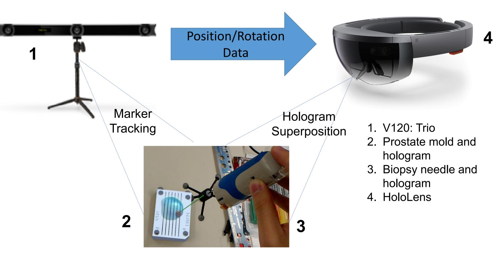
Figure 3. Schematic overview of the system setup
