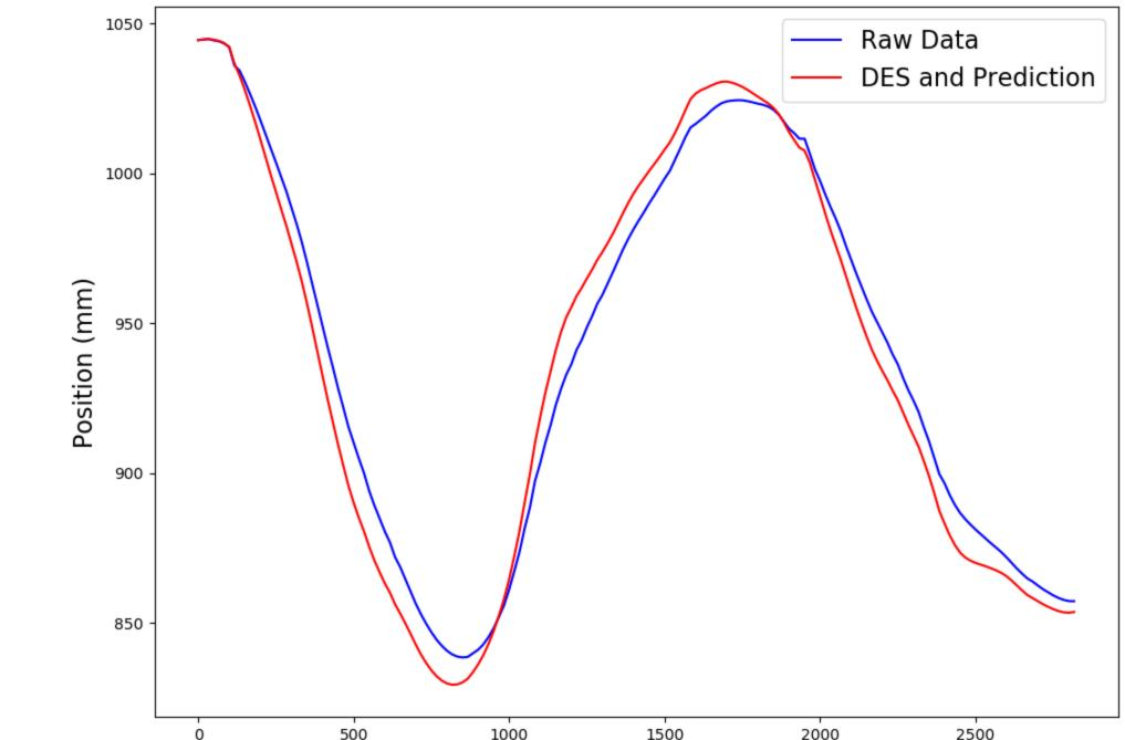
Figure 5. Example of double exponential smoothing and prediction for z position. Smoothing and prediction are applied to x, y, and z position, as well as to the quaternion. This example shows a 50 ms future prediction, used to reduce visual hologram latency.
