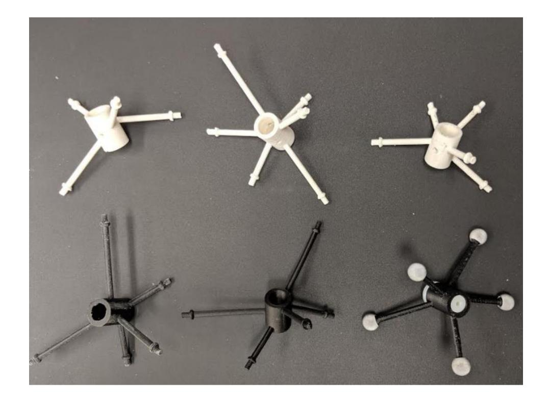
Figure 2. Marker configuration designs for the biopsy needle. Important parameters include marker size, separation, and orientation.
