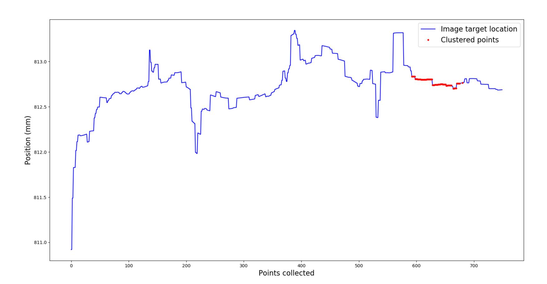
Figure 4. Example density-based clustering results for z position. Our implementation uses both positional and rotational data to find the most dense cluster of points, which represents alignment of the hologram and image target. This data is used to synchronize the V120: Trio and HoloLens coordinate systems.
